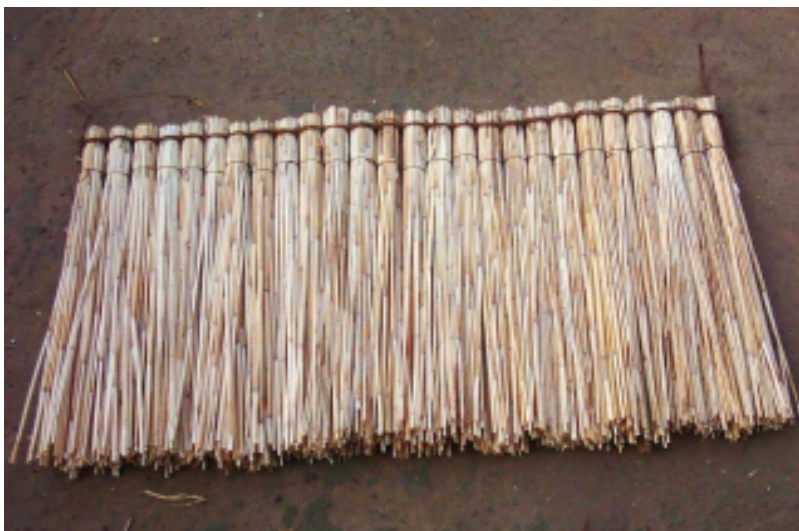
Plate 7: The Example of a Thatch Materials Used In Roofing.
