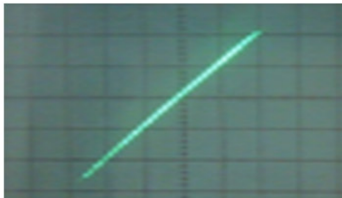
Fig. 7: Complete synchronization of coupled Non-Identical and Periodically Forced \phi^6 -Duffing and \phi^6 -Van der Pol circuits for R_C = 1m\Omega .
