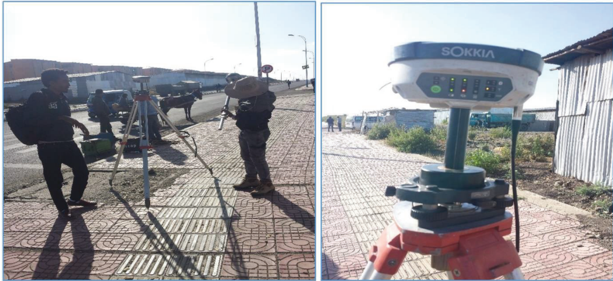
Figure 2.5: RTK-DGPS adjustment at the base station (left) and the adjusted base station (Receiver) (right)
