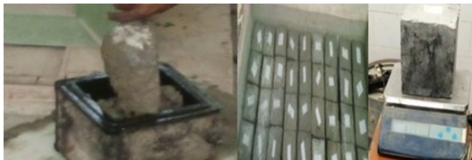
Figure 9 Casting, compacting, curing, weighting, and breaking of cubes
