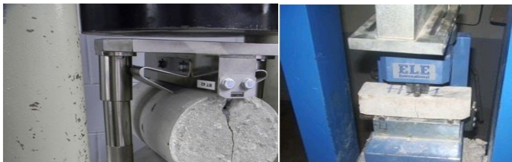
Figure 4: tensile strength tests on cylindrical and cubic specimens
