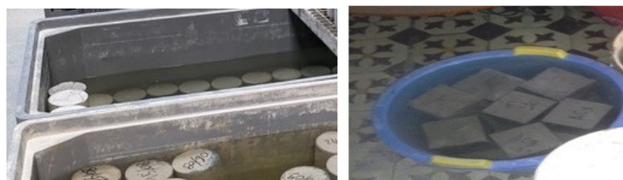
Figure 2: preservation of test specimens in water
