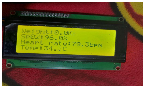
Figure 10. Result Obtained by the Sensors on LCD during Experiment 2
