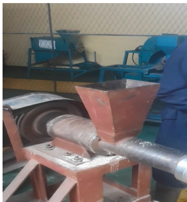
Fig 5: The modified extruder dies and tested with maize with wheat ingredient
