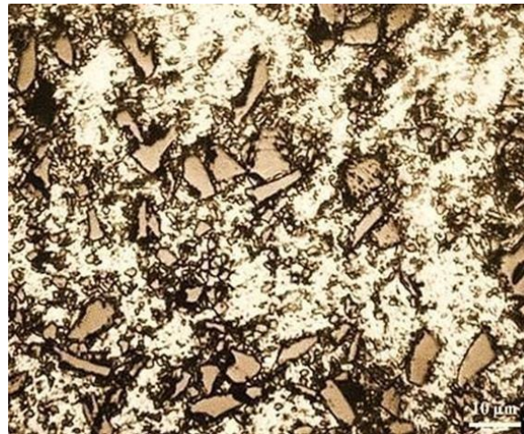
Figure 1. The microstructure of the as-extruded sample with 37 vol. % reinforcement.
