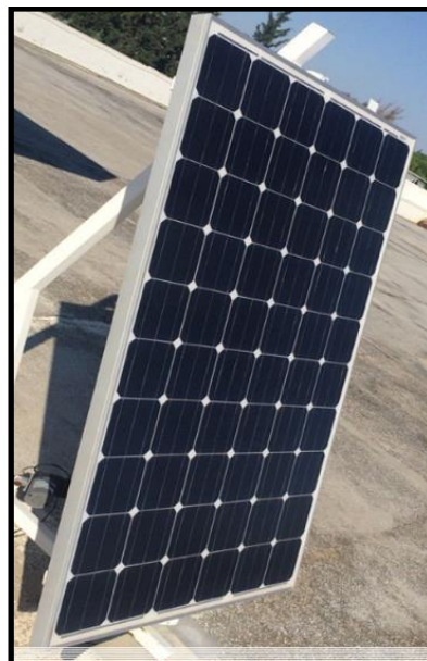
Figure 2. Vertical axis STS with PV module and step motor
