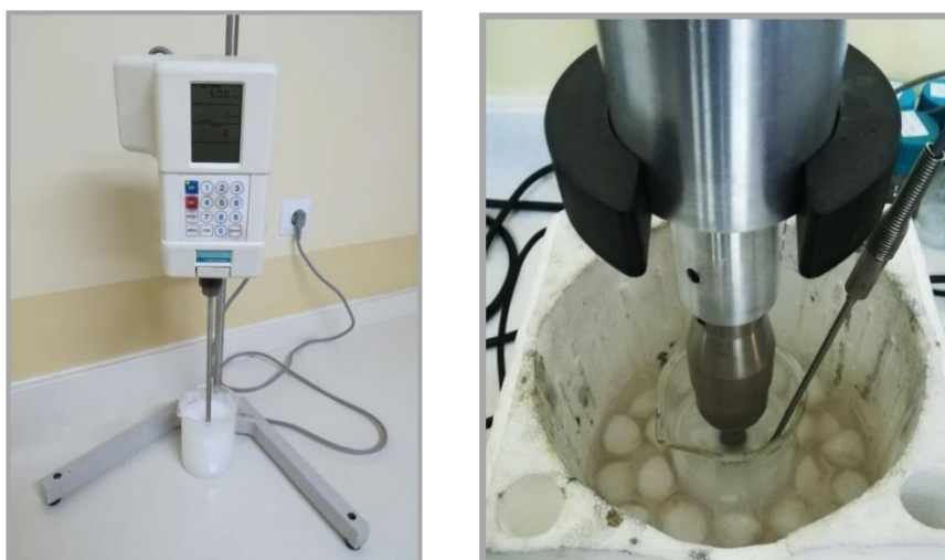
Figure 1.a. Preparation of nanoparticles b. cold water bath is used for temperature control.
