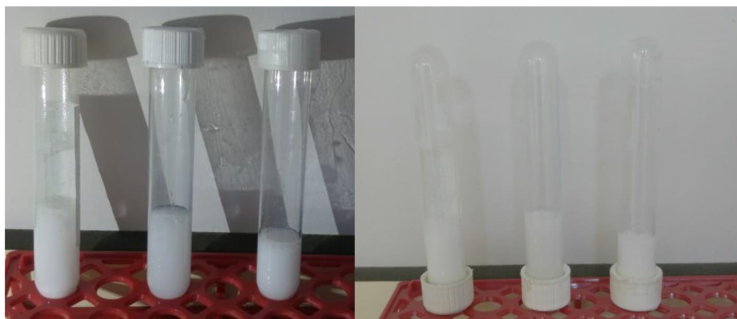
Figure 1. Photographic image of \text{TiO}_2 , \text{Al}_2\text{O}_3 and \text{TiO}_2\text{-Al}_2\text{O}_3 nanoparticles in water, from left to right respectively.
