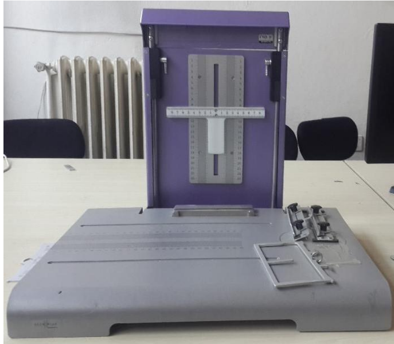
Figure 3. The test tool for stretching and slipping tests.
